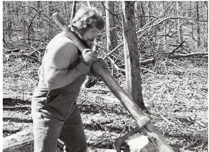
Terry is using a cant hook—a tool to move logs. It consists of a sturdy wooden handle that works like a lever, with a movable iron hook that is snugged into the log to hold it in place. He’s trying to roll the log over so it can be cut with the crosscut saw from the other side.
