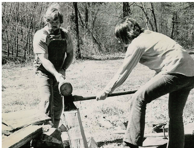
Terry and Bob Goodwin work together to split some of the white oak logs into chunks suitable for shingle-making using a hickory maul and an axe as the wedge.
